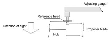
Now the angle gauge touches the lower side of the profile of the propeller blade at one point. Turn the blade until the back edge of its profile and another point of the frontal profile area of the blade touch the tongue of the adjusting gauge. Now a specified angle is established (sketch).
